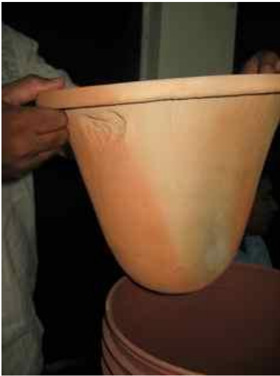
Example of a ceramic filter from Plan International similar to the Potters for Peace filters used in the village. This one has a different shape and is not impregnated with silver.
