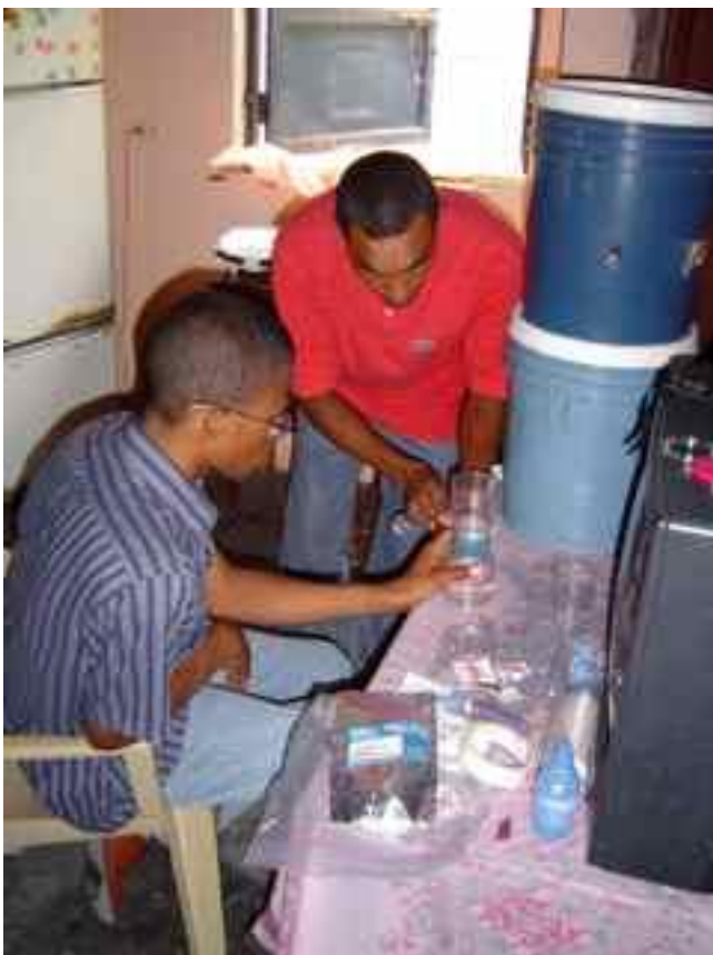
Testing water from a two-stage bucket filter for fecal coliform in June 2006.
